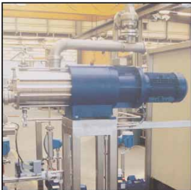
Installation of Pentax Multi-Frequency Fluid Mixer.
