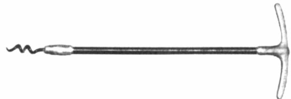
Figure 4-2. Packing Removal Tool
