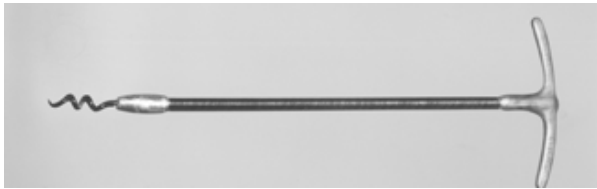
Figure 4-2. Packing Removal Tool
